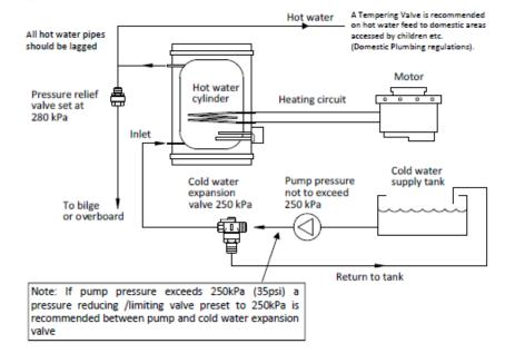
Larger sizes of 110–1000 litres are made with a working pressure of 500kPa can be made to order with a stainless steel inner barrel and outer case. Heating coils can also be incorporated in the larger sized marine cylinders to utilise excess heat from the vessel's engine heat exchanger. 1kW booster element or larger are available on request.
